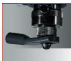
Vacuum nose 3.3 mm diameter Part No. 21672
