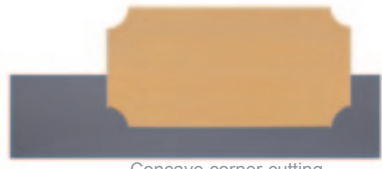
Concave corner cutting For up to 40 mm width For up to 80 mm width
